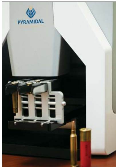
A central component of the ALIAS system from Pyramidal Technologies Ltd. is the interferometer. The device captures light-independent images of both bullets and cartridge cases based on highly detailed measurements.
