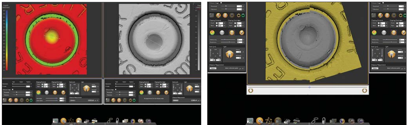
The interactive visualization interface provided by Pyramidal Technologies' ALIAS can render images of bullets or cartridge cases in natural color, grey-scale, or topographically sensitive color, and allows users to easily switch between these views. The image on the left shows two cartridge cases with their primer areas. On the right, the images of two cartridge cases are merged to aid in comparison and prove a match. An examiner can split two cartridge images vertically and slide them together to determine if the halves match.
