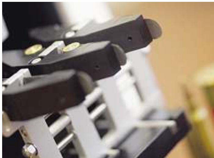
HIGH PRECISION: A Swiss-built interferometer scans the surface of the expended cartridge cases with a six-pack cartridge case holder
