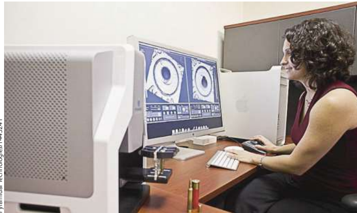
TEST SITE: The ALIAS system creates a digital clone of a fired bullet
